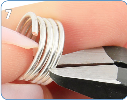
7. Alternate cutting the coiled wire into single rings using the flush side of cutters. The ends should meet flush.
